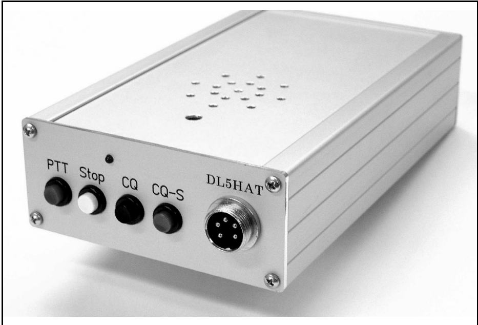
Fig 2 : Completed speech store in an aluminium case as produced by Frank Peter Richter, DL5HAT.
